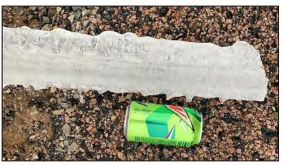
Ice in some areas was up to 3 to 4 inches on power lines, causing massive destruction when facing the adverse weather conditions, including high winds that snapped the heavy power lines. (Left photo by Glen Fogle, a WFEC lead power line technician - top photo from CKenergy Electric Cooperative, which suffered extensive damage across their service area).
